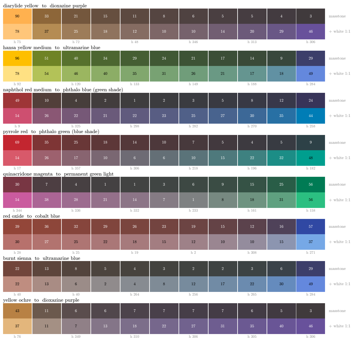
Figure 24: Eight pairs from across the hue circle, mixed in steps of ten percent by weight, in masstone and with an equal weight of white, as in Figure 23. The pairs pass through gray where the two reflectances no longer overlap.
