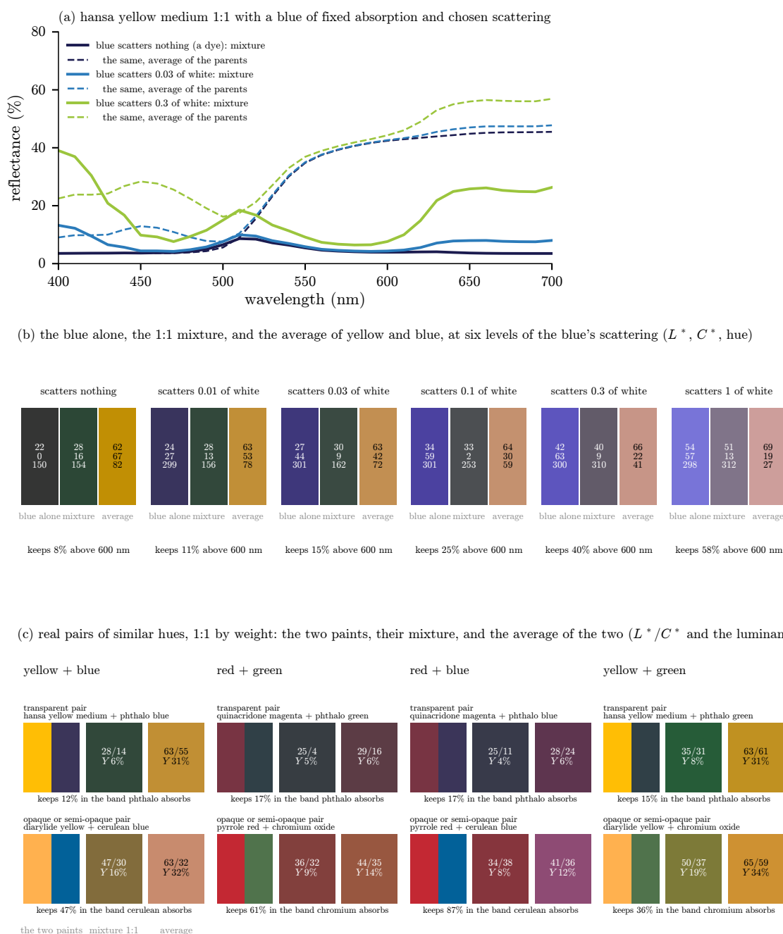
Figure 14: Between subtracting and adding. (a) Hansa yellow medium mixed half and half with an imaginary blue that absorbs like phthalo blue, given three amounts of scattering; the dashed curves are the plain averages of the two paints, the fully additive case. (b) The same at six amounts of scattering: the blue alone, the mixture, the average, and the share of the average's light the mixture keeps where the blue absorbs. (c) Four real pairs of similar hues, each made once from transparent or semi-transparent paints and once from opaque or semi-opaque ones by Golden's ratings, half and half by weight, with the same comparison.
